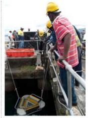
Participants lower a disc skimmer that will separate oil from seawater and pump the oil into inflatable tanks.
