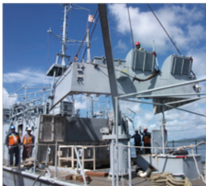
The Kikau II superstructure was removed to give access to the systems needing repair.
